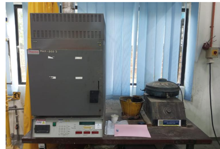
Furnace & Asphalt centrifuge
